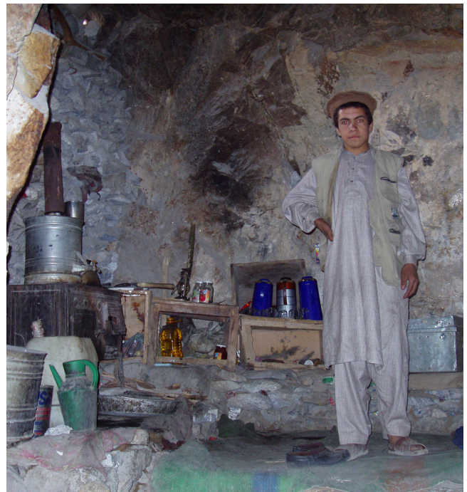
Old mine adits like this one are used as living quarters complete with sleeping areas and kitchens. Note that smoke from the cooking stove is not vented outside of the mine. Gary Bowersox photo.
