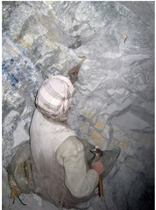
After holes are drilled next to the lapis veins they are loaded with explosives to break up the enclosing rock. Bilal Afridi photo.
